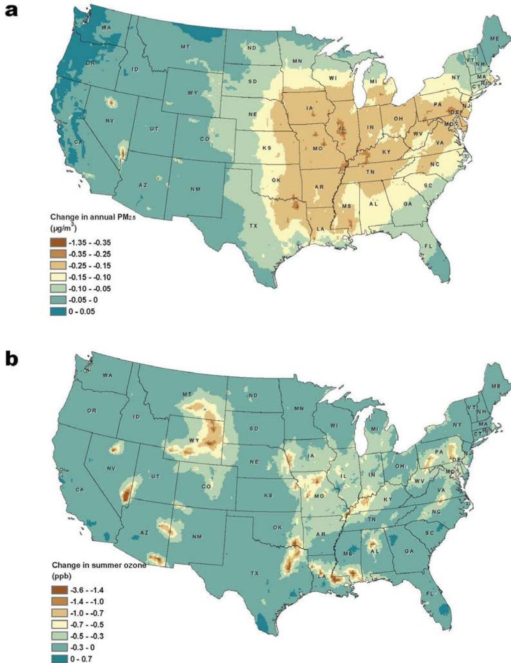
**Supplementary Figure 1.** Maps for the continental U.S. of difference in annual average concentrations of fine particulate matter (PM<sub>2.5</sub>) in micrograms per cubic meter (a) and the difference in annual average concentrations of peak summertime ozone in parts per billion (b) for Scenario 3 less the reference scenario in 2020.
